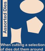
When cutting a selection of dies dot them around the plates rather than placing in a uniform way to ease the pressure.
