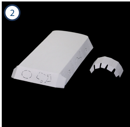
2. Fold along the score lines of the A and B die cuts as shown.
