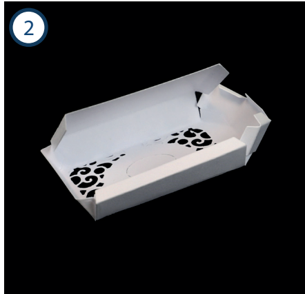
2. Valley fold along all the score lines of the A die cut.
