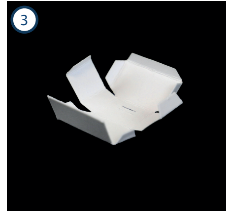
3. Valley fold along all the score lines of the C die cut. Secure by sticking the tabs to the corresponding sides.
