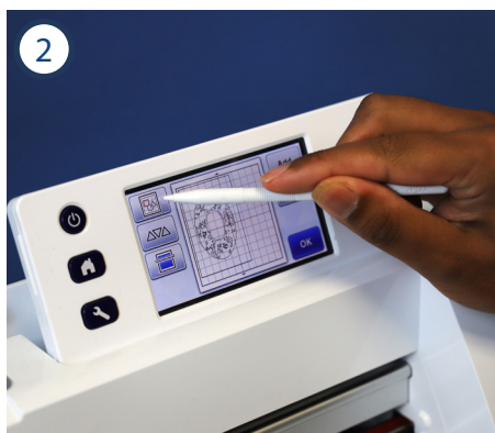
Open the file on the Scan N Cut and go into the Edit menu.
